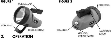
A three-position switch (spotlight, off, area light) controls on/off operation of both lights. The spotlight can be continuously lit for up to 25 minutes on a full battery charge. The area light can be lit for up to 15 hours on a full battery charge. The unit may be operated during DC recharge only. Figure 1 shows locations of the handle, adjustable stand. Figure 2 rear view, shows spotlight/off/area light switch, area light and handle lock button.
